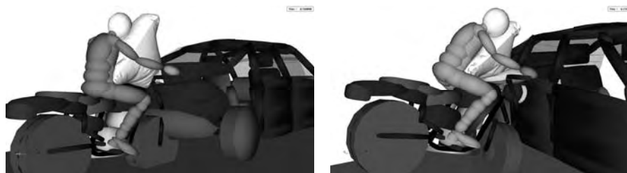
Figure 10a, 10b: Computational simulation with airbag (2.Generation), deformation structure, Knee airbag in impact configuration 711 and 413 according to ISO 13232
