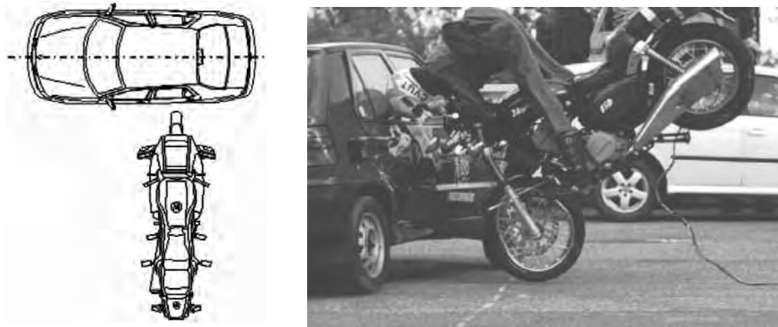
Figure 8a, 8b: Experimental simulation in impact configuration 413 according to ISO 13232 [2]
