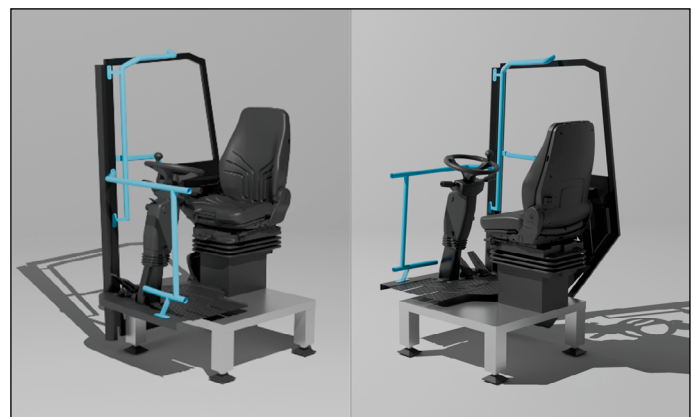
Fig. 2 The vehicle simulator platform visualization.
